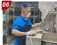
Build Mould Shell
